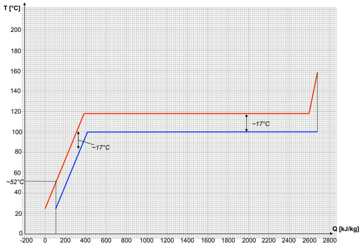
The minimum approach temperature is around 17°C both during the boiling/condensing phase and the liquid exchange phase. In both cases, we are well above the recommended minimum approach temperature making this process completely feasible. Notice that there is no true pinch point here because we have too much heat at high temperature!
